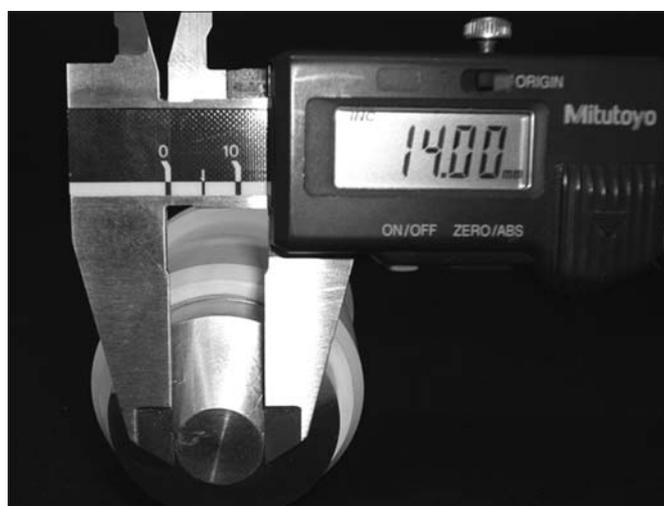
**Figure 3.** Reduced headstock of therapeutic ultrasound (14mm).
