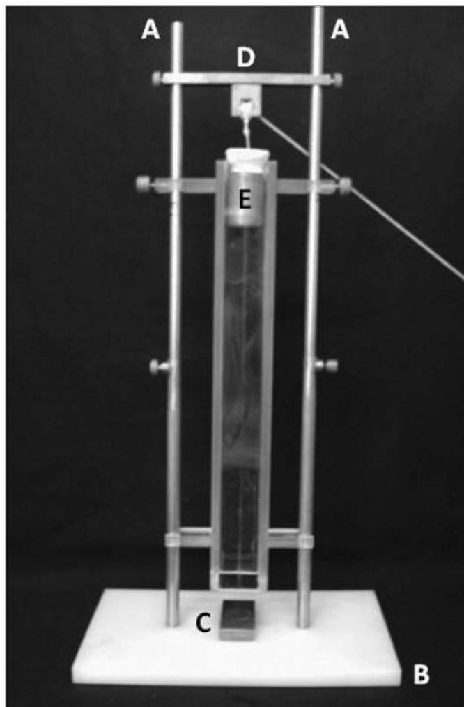
**Figure 1.** Equipment of production of the experimental lesion composed by two adjustable metallic stems from 30 to 40cm (A), plastic base with 272.5cm<sup>2</sup> of area (B), rectangular metallic surface with 12.25cm<sup>2</sup> of area (C) and metallic structure that supports the pulley (D) and a thread connect to a mass of 200g close to be liberated (E).
