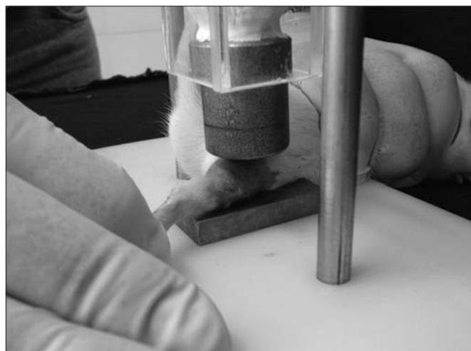
**Figure 2.** Equipment of production of the experimental lesion when the mass of 200g falls in the middle of gastrocnemius muscle.
